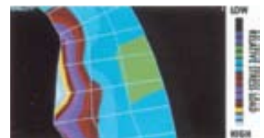
Wright Drive. The Wright Drive distributes stress evenly across the socket and fastener faces, away from the fastener corners, and over a larger flat contact area than ordinary sockets allow. There is a significant improvement in distribution of stress at the socket's inside surface.
